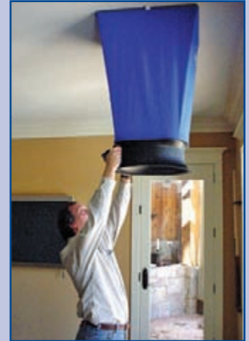
Air-flow testing ensures that the home's comfort meets the standards set during the design process.
